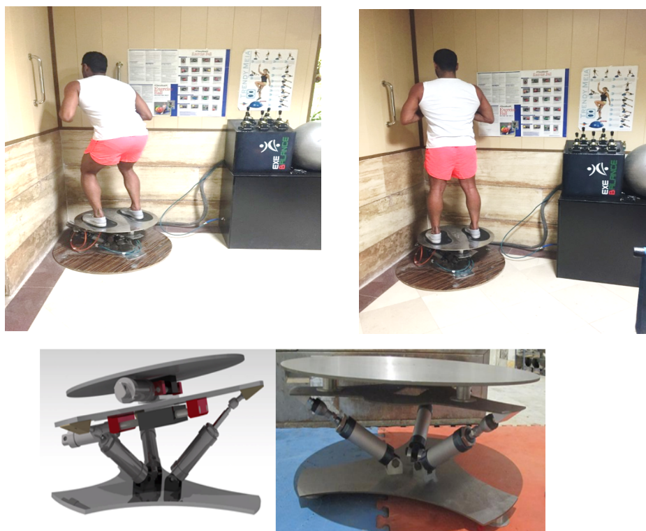
Figure 1. The general panel of the exe-balance device, the perturbation plate, and two protective handles mounted on the wall to hold. The right picture shows a participant standing on the perturbation plate while flexing his knees to achieve more stability. The left image shows a standby participant standing with extended knees on the plate.
