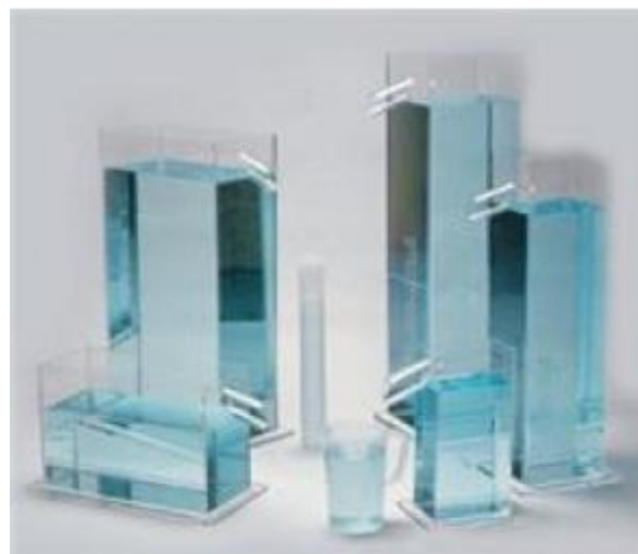
Figure 1. A volumeter to measure limb volume by water displacement
