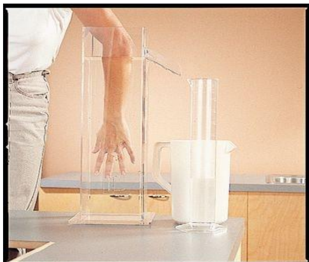
Figure 2. The arm was placed in a water-filled cylinder (volumeter) and the overflowing water was measured
