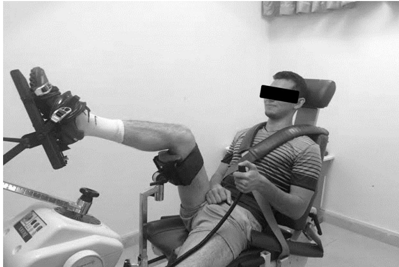
Figure 2. Joint position sense testing using Biodex isokinetic dynamometer
